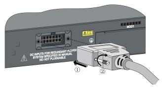
Step5 Connect the other end of the +12 VDC RPS power cord to the external RPS power supply system.
